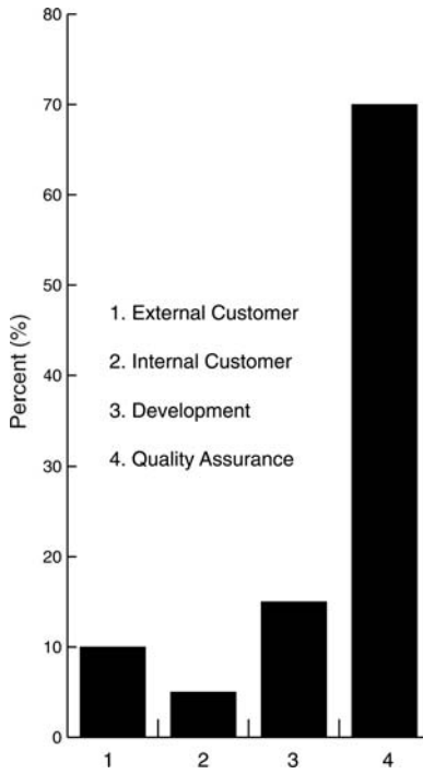
Exhibit 20.9. Defects by Who Found
